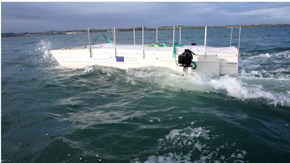
Figure 4 - GKinetic CEFA 12 Tow Testing demonstrating stability @ 2.5m/s
